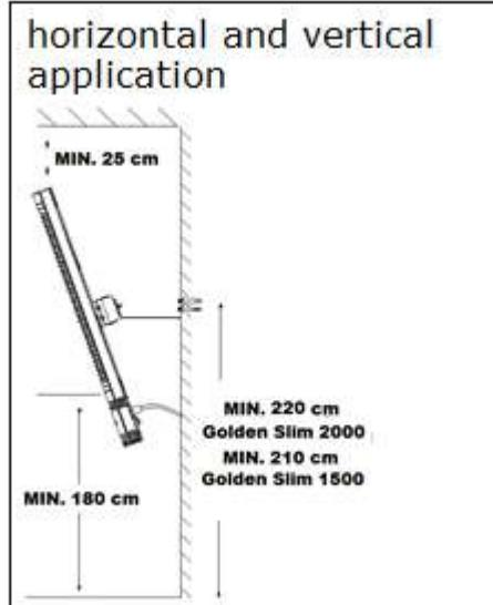
The Golden Slim infrared heater is equipped with a rotatable wall bracket so that it can be used horizontally or vertically. This deserves special attention when installing the appliance, because you must take into account the minimal distances from the wall, ceiling and ground in all the optional positions:
